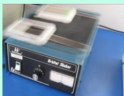
All incubation steps must be performed on an orbital shaker with 18+ mm orbital diameter
