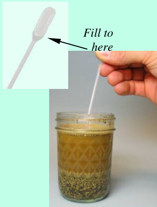
Avoid pulling up particles when drawing sample
