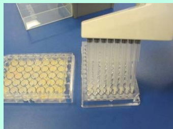
Add Enzyme-Conjugate, followed immediately by Control and sample extracts, to the plate
